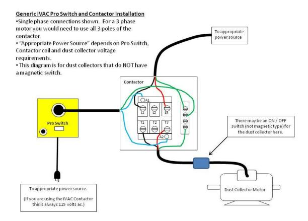
Place the power cable that will bring power from the source to the dust collector through the chosen gland and secure it by tightening the gland cover nut. Connect the green ground wire in this cable to the ground bar in the bottom of the contactor enclosure.
