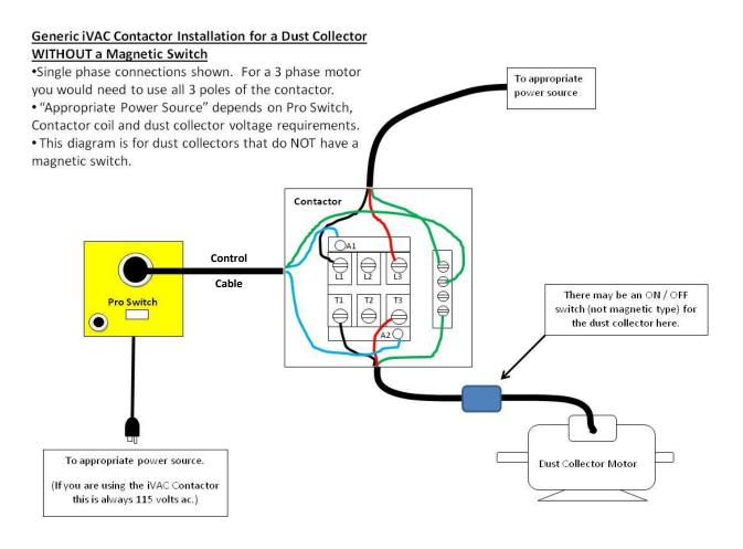
Place the power cable that will bring power from the source to the dust collector through the chosen gland and secure it by tightening the gland cover nut. Connect the green ground wire in this cable to the ground bar in the bottom of the contactor enclosure.
